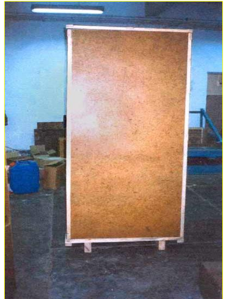
Totally closed Coir Composite Board sheathed Crate for the Circuit breaker
