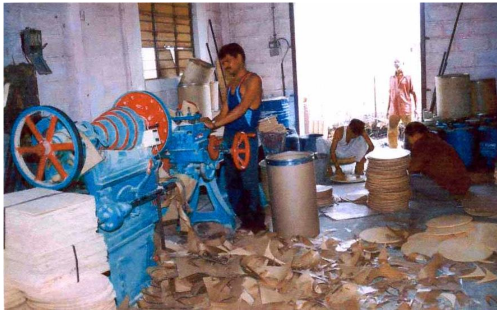
Circular cutting of lids for fibre drums
